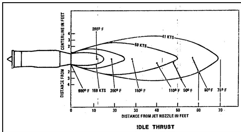
Figure 7.--JT8D turbofan exhaust gas temperatures and velocities.
